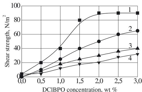
Fig. 4. Effect of DCIBPO concentration on shear strength of silicone PSA at different temperatures: 1 — 20 °C, 2 — 70 °C, 3 — 120 °C, 4 — 180 °C
