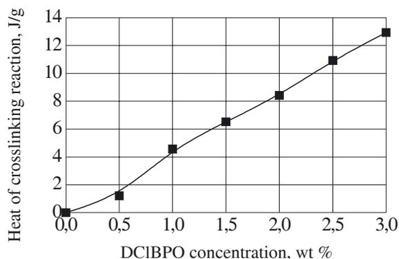
Fig. 2. Effect of DCIBPO concentration on the heat of crosslinking reaction of silicone PSA
