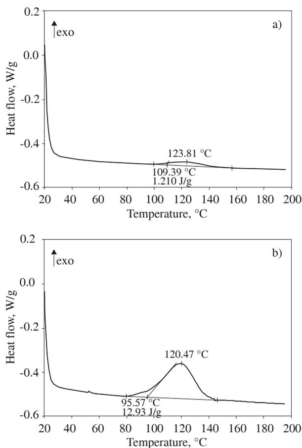
Fig. 1. Thermodynamic characteristic of silicone PSA crosslinking process catalyzed by: a) 0.5 wt. % of DCIBPO, b) 3.0 wt. % of DCIBPO
