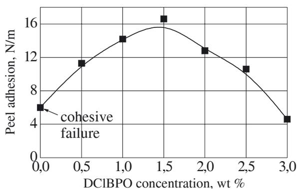
Fig. 3. Effect of DCIBPO concentration on peel adhesion of silicone PSA
