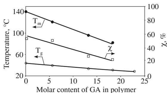
Fig. 4. Melting temperature ( $T_m$ ), glass transition temperature ( $T_g$ ) and degree of crystallinity ( $\chi$ ) determined by DSC as functions of molar content of GA in polymers
