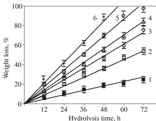
Fig. 5. Weight loss of PLLA (1), PLLAc (2) and PLLGAc (3—6) oligomers
