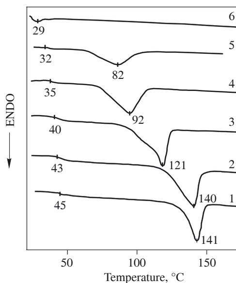
Fig. 3. DSC thermograms of PLLA (1), PLLAc (2) and PLLGAc (3—6) oligomers
