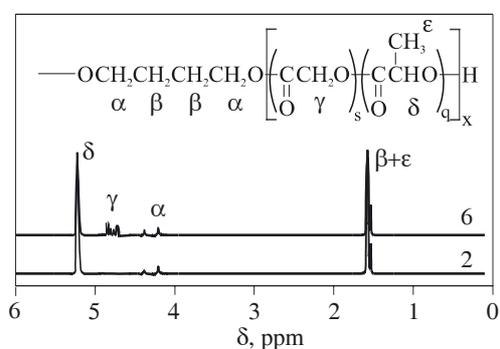
Fig. 2.  $^1\text{H}$  NMR spectra of PLLAc (2) and PLLGAc-80 (6) oligomers
