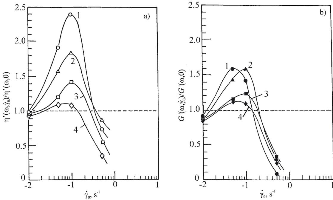
Fig. 7. Influence of the superposed shear rate ( $\dot{\gamma}_0$ ) on: a) dynamic viscosity ( $\eta'$ ) and b) storage modulus ( $G'$ ) normalized by their values from simple oscillatory flow for CF20/PE system at various angular frequencies ( $\omega$ ): 1 — 0.6 rad/s, 2 — 1.6 rad/s, 3 — 6 rad/s, 4 — 20 rad/s
