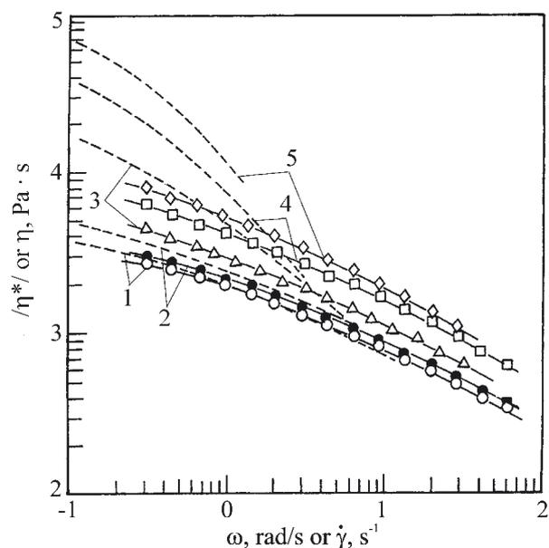
Fig. 1. Relationship between complex viscosity ( $|\eta^*|$ ) and angular frequency ( $\omega$ ) of unfilled PE-LD and CF/PE-LD melts. Particular samples are denoted as follows: 1 — PE, 2 — CF5/PE, 3 — CF10/PE, 4 — CF15/PE, 5 — CF20/PE; broken lines represent shear viscosity ( $\eta$ ) versus shear rate ( $\dot{\gamma}$ )
