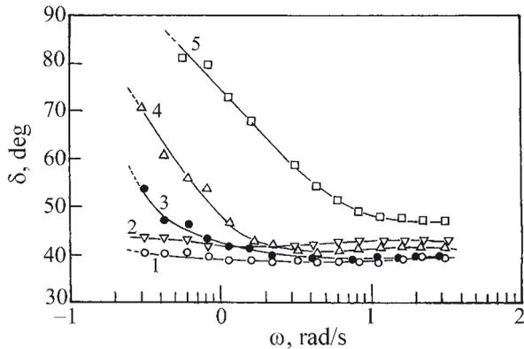
Fig. 11. Influence of angular frequency ( $\omega$ ) on phase angle ( $\delta$ ) for CF20/PE system; parameter, the superposed shear rate ( $\dot{\gamma}_0$ ), changes as: 1 —  $0 \text{ s}^{-1}$ , 2 —  $0.01 \text{ s}^{-1}$ , 3 —  $0.05 \text{ s}^{-1}$ , 4 —  $0.1 \text{ s}^{-1}$ , 5 —  $0.5 \text{ s}^{-1}$
