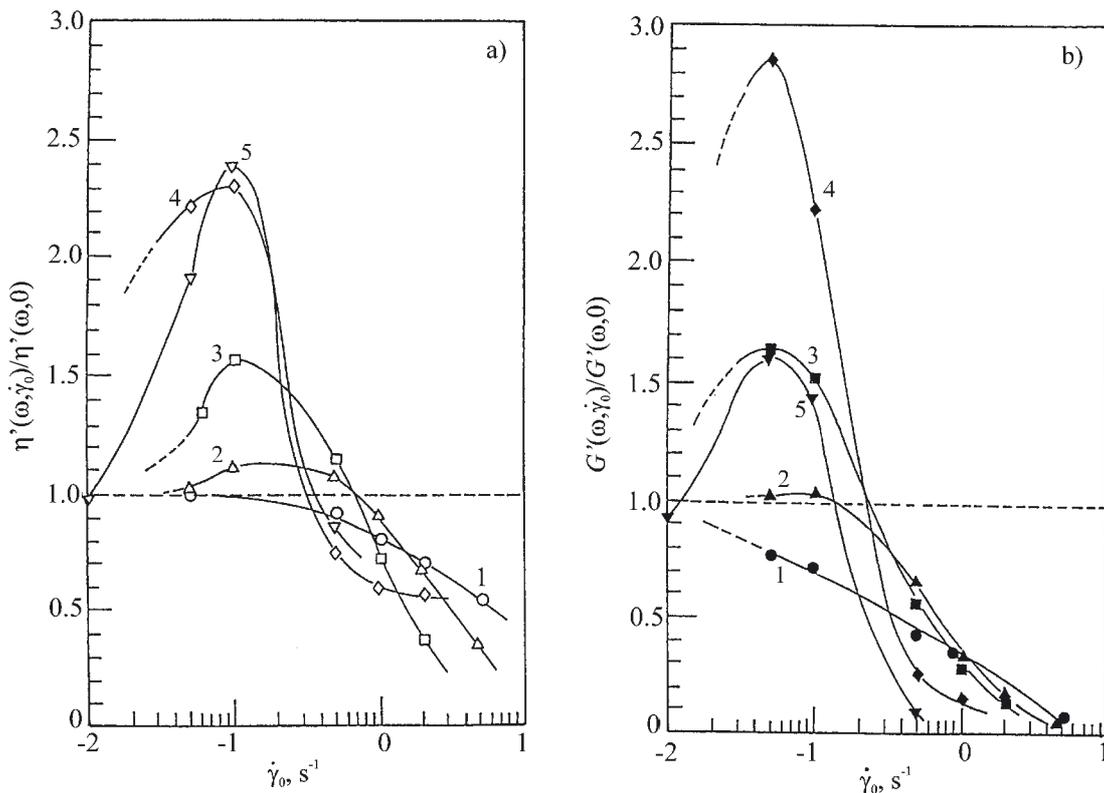
Fig. 8. Influence of the superposed shear rate ( $\dot{\gamma}_0$ ) on: a) dynamic viscosity ( $\eta'$ ) and b) storage modulus ( $G'$ ) normalized by their values from simple oscillatory flow for unfilled PE sample and CF/PE melts at the angular frequency of 0.6 rad/s; particular samples are denoted as follows: 1 — PE, 2 — CF5/PE, 3 — CF10/PE, 4 — CF15/PE, 5 — CF20/PE
