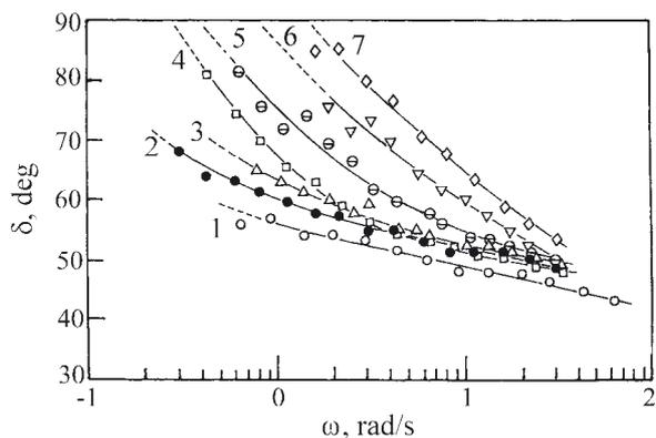
Fig. 4. Phase angle ( $\delta$ ) versus angular frequency ( $\omega$ ) curves of unfilled PE sample; parameter, the superposed shear rate ( $\dot{\gamma}$ ), changes as: 1 —  $0 \text{ s}^{-1}$ , 2 —  $0.05 \text{ s}^{-1}$ , 3 —  $0.1 \text{ s}^{-1}$ , 4 —  $0.5 \text{ s}^{-1}$ , 5 —  $1 \text{ s}^{-1}$ , 6 —  $2 \text{ s}^{-1}$ , 7 —  $5 \text{ s}^{-1}$
