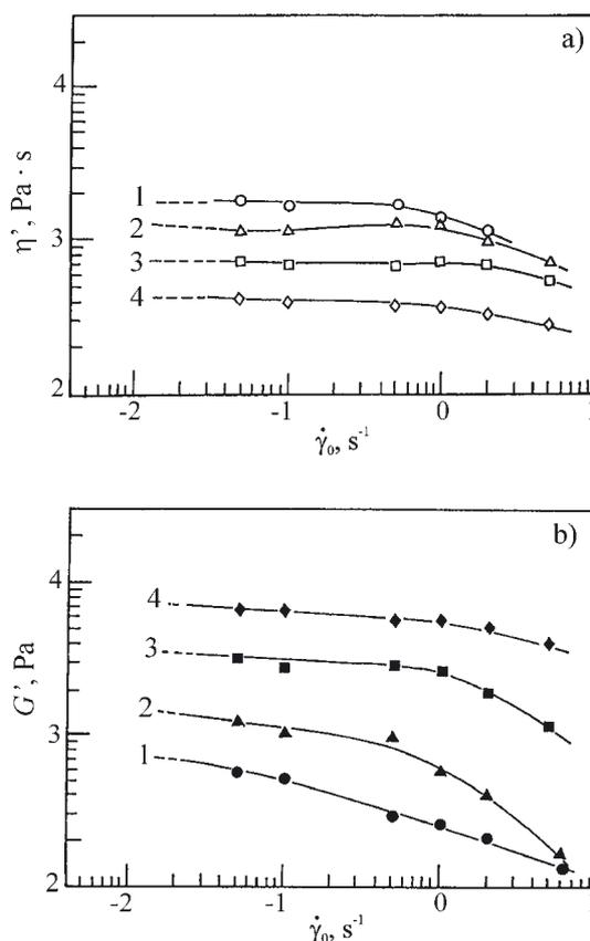
Fig. 3. Influence of superposed shear rate ( $\dot{\gamma}_0$ ) on: a) dynamic viscosity ( $\eta'$ ) and b) storage modulus ( $G'$ ) for unfilled PE sample at various angular frequencies ( $\omega$ ): 1 —  $0.6 \text{ rad/s}$ , 2 —  $1.6 \text{ rad/s}$ , 3 —  $6 \text{ rad/s}$ , 4 —  $20 \text{ rad/s}$
