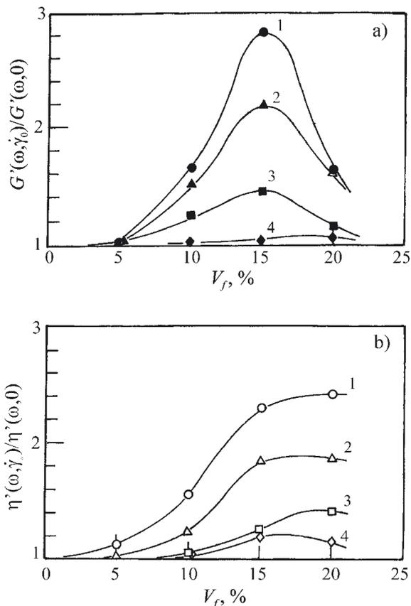
Fig. 10. Influence of volume fraction of fibre ( $V_f$ ) on: a) maximum storage modulus ( $G'_{max}$ ) and b) maximum dynamic viscosity ( $\eta'_{max}$ ) normalized by their values from simple oscillatory flow at various angular frequencies ( $\omega$ ): 1 — 0.6 rad/s, 2 — 1.6 rad/s, 3 — 6 rad/s, 4 — 20 rad/s
