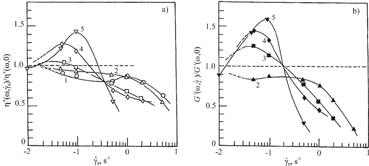
Fig. 9. Influence of the superposed shear rate ( $\dot{\gamma}_0$ ) on: a) dynamic viscosity ( $\eta'$ ) and b) storage modulus ( $G'$ ) normalized by their values from simple oscillatory flow for unfilled PE sample and CF/PE melts at the angular frequency of 6 rad/s; particular samples are denoted as follows: 1 — PE, 2 — CF5/PE, 3 — CF10/PE, 4 — CF15/PE, 5 — CF20/PE
