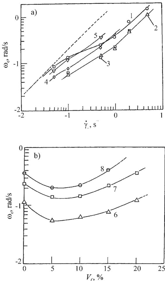
Fig. 12. Critical angular frequency ( $\omega_c$ ) for unfilled PE sample and CF/PE melts as a function of: a) superposed shear rate ( $\dot{\gamma}_0$ ) for: 1 — PE, 2 — CF5/PE, 3 — CF10/PE, 4 — CF15/PE, 5 — CF20/PE systems (broken line represents  $\omega_c = \frac{1}{2}\dot{\gamma}_0$  relationship); b) volume fraction of fibre ( $V_f$ ) for shear rate ( $\dot{\gamma}$ ) varied as 6 —  $0.1 \text{ s}^{-1}$ , 7 —  $0.5 \text{ s}^{-1}$ , 8 —  $1 \text{ s}^{-1}$
