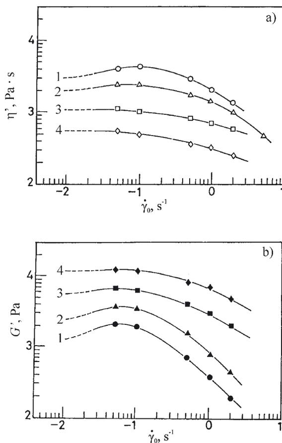
Fig. 6. Influence of superposed shear rate ( $\dot{\gamma}_0$ ) on: a) dynamic viscosity ( $\eta'$ ) and b) storage modulus ( $G'$ ) for CF10/PE system at various angular frequencies ( $\omega$ ): 1 —  $0.6 \text{ rad/s}$ , 2 —  $1.6 \text{ rad/s}$ , 3 —  $6 \text{ rad/s}$ , 4 —  $20 \text{ rad/s}$
