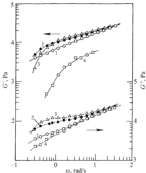
Fig. 5. Storage and loss moduli ( $G'$ ,  $G''$ ) versus angular frequency ( $\omega$ ) curves of CF20/PE system; parameter, the superposed shear rate ( $\dot{\gamma}$ ), changes as: 1 —  $0 \text{ s}^{-1}$  (0 Pa), 2 —  $0.05 \text{ s}^{-1}$  ( $54 \cdot 10^2 \text{ Pa}$ ), 3 —  $0.1 \text{ s}^{-1}$  ( $80 \cdot 10^2 \text{ Pa}$ ), 4 —  $0.5 \text{ s}^{-1}$  ( $120 \cdot 10^2 \text{ Pa}$ ); the data given in brackets represent values of corresponding shear stress
