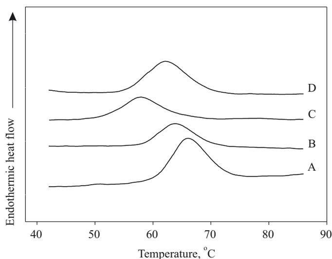
Fig. 9. DSC thermograms of the starch borated with boric acid (B) and borax (C) (starch:borating agent = 1:1) at 450 W for 1800 s; potato starch prior (A) and after (D) heating under identical conditions are added for comparison
