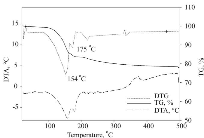
Fig. 3. Thermogram of boric acid
