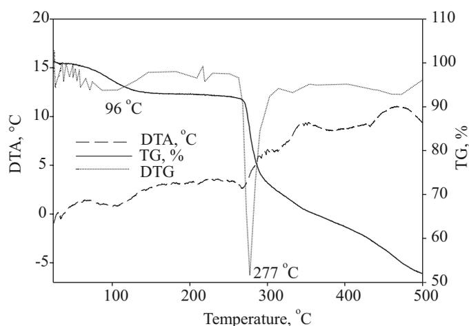
Fig. 2. Thermogram of potato starch
