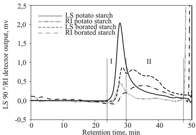
Fig. 1. An example of superimposed chromatograms of RI and LS  $90^\circ$  detector outputs for starch borated with boric acid (starch:boric acid = 1:0.1) at 450 W and for 1800 s (see text); chromatograms for the potato starch are shown for comparison
