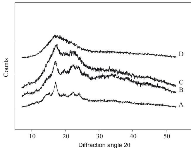
Fig. 12. Powder X-ray diffraction patterns of the starch borated with boric acid (B) and borax (C) (starch:borating agent = 1:1) at 800 W for 1800 s; potato starch patterns prior (A) and after (D) heating under identical conditions are added for comparison
