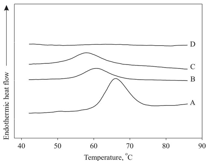
Fig. 10. DSC thermograms of the starch borated with boric acid (B) and borax (C) (starch:borating agent = 1:1) at 800 W for 1800 s; potato starch diagrams prior (A) and after (D) heating under identical conditions are added for comparison
