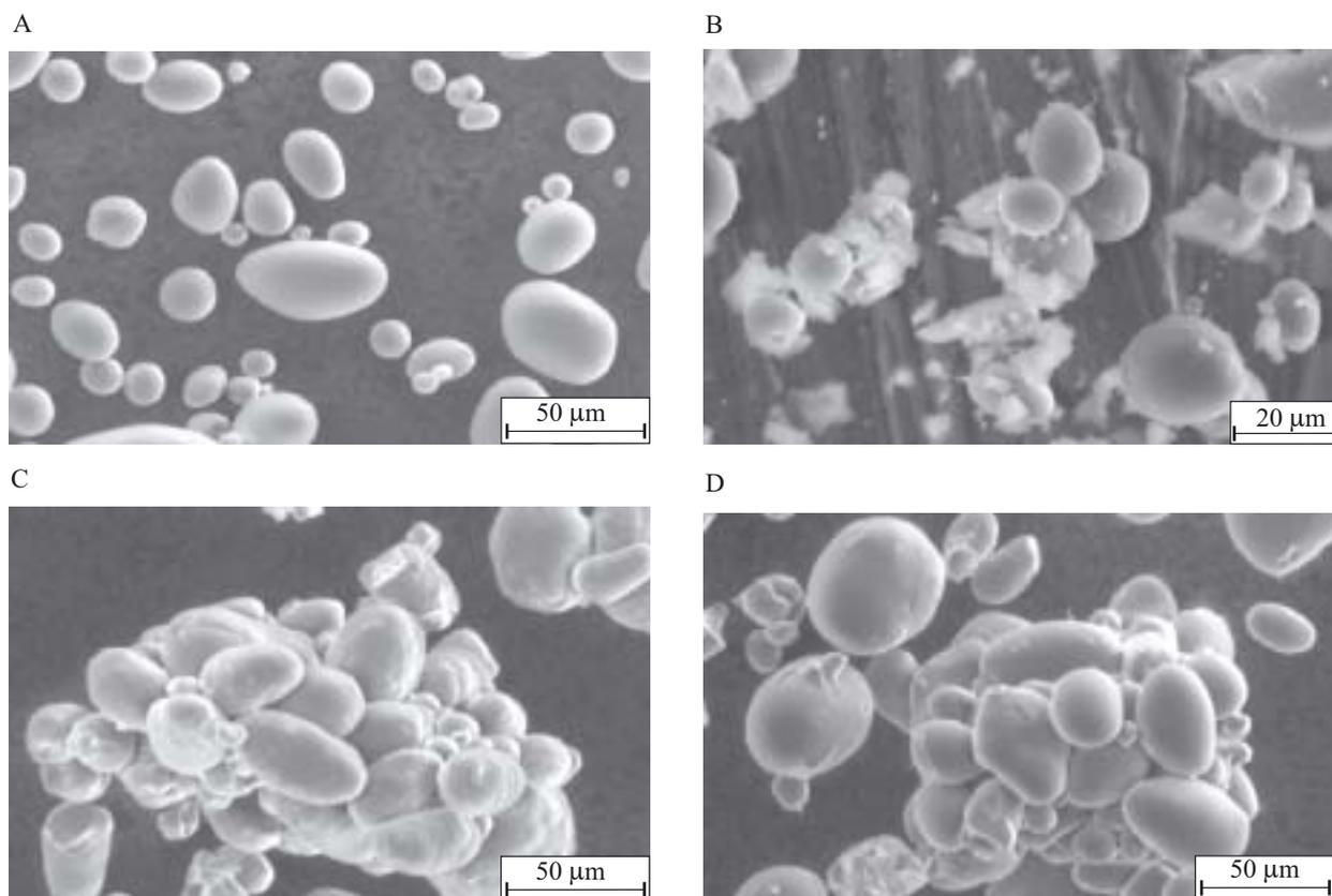
Fig. 13. SEM images of potato starch prior (A) and after (B) microwave radiation at 800 W for 1800 s, and of the starch borated with boric acid (C) and borax (D) (starch:borating agent = 1:1) under the same heating condition
