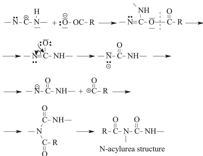
Scheme A. Mechanism of the reaction between carboxylic groups and polycarbodiimides during crosslinking of acrylic PSAs
