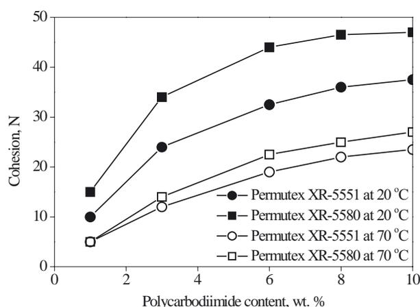
Fig. 2. Effect of kind and amount of crosslinking agent on the acrylic PSA cohesion
