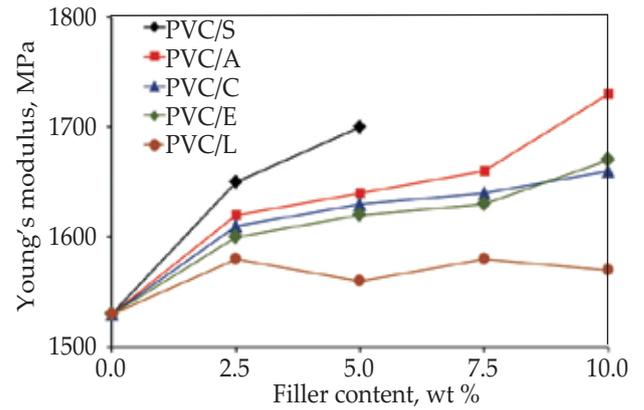
Fig. 5. Young's modulus of PVC and PVC-based composites vs. filler content: silica, lignin, and lignin/silica fillers in weight ratios of 1 : 5, 1 : 1 and 5 : 1 wt/wt
