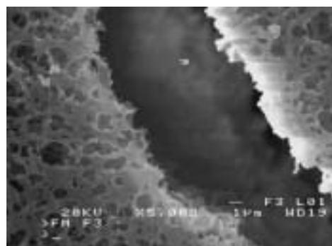
Fig. 6. SEM image of the fracture surface of crack in the membrane wall observed in the samples after 171 h periodic MD process of NaCl solutions
