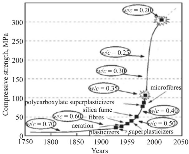
Fig. 1. Generalized curve of concrete development [3]
