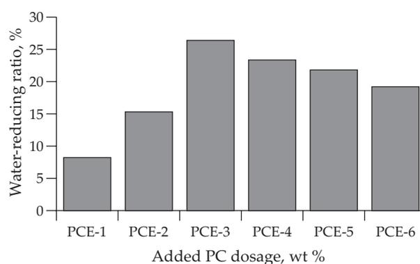
**Fig. 3.** Effect of carboxylic groups content in PCE on the fluidity at the  $w/c$  ratio of 0.24 (left) and the water-reducing ratios, dosage: 0.2 wt % by cement weight (right) [14]**Table 5.** PCE concentration to reach a paste flow of  $26 \pm 0.5$  cm in the “mini slump” test [48]
