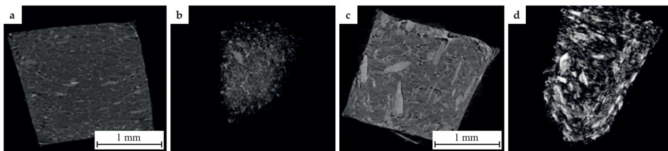
Fig. 5. Thermographic images of the composites: a) 2D for PE-S15, b) 3D for PE-S15, c) 2D for PE-P30, d) 3D for PE-P30
