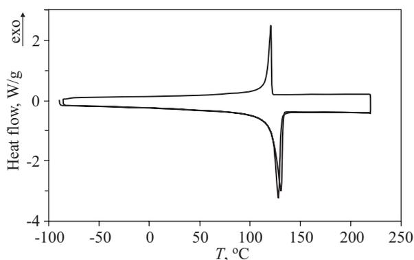
**Fig. 2.** DSC curves of PE-S5 composite**Table 4.** The density of the composites (the values in parentheses are the standard deviations)
