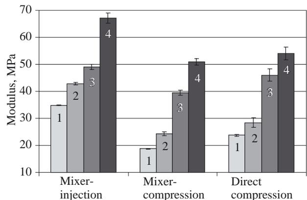
Fig. 6. Influence of compounding processes on tensile and flexural strength of abaca fibre-PP composites (fibre length: 5 mm, fibre content: 30 wt. %): 1 — tensile strength, without MAH-PP; 2 — tensile strength, with 5 wt. % of MAH-PP, 3 — flexural strength, without MAH-PP; 4 — flexural strength, with 5 wt. % of MAH-PP
