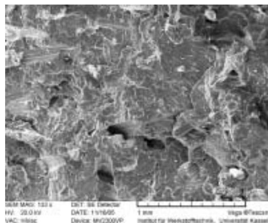
Fig. 2. Influence of coupling agent MAH-PP on the microstructure of abaca fibre-PP composite with 5 mm fibre lengths in injection molding process (fibre content: 30 wt. %)
