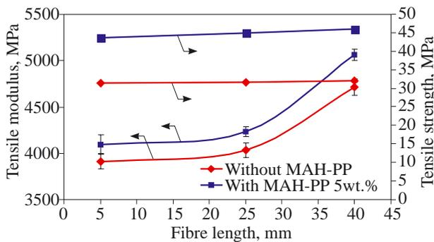
Fig. 4. Influence of fibre length on tensile modulus and strength of abaca fibre-PP composites in injection molding process (fibre content: 30 wt. %)
