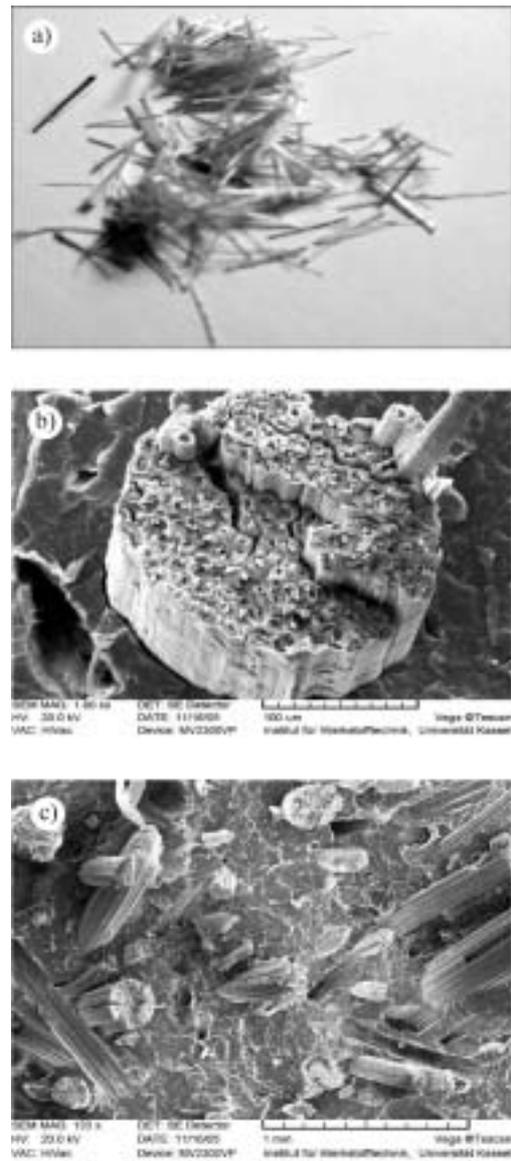
Fig. 1. Raw abaca fibre, SEM micrographs of it and of fibre in PP composite obtained by injection molding process: a) raw fibre, b) cross-section of fibre, c) fibre in composite (fibre content 30 wt. %, fibre length 5 mm)
