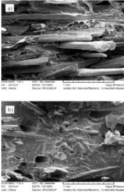
Fig. 3. Influence of MAH-PP on the microstructures of abaca fibre-PP composites in direct compression molding process: a) without MAH-PP, b) with 5 wt. % of MAH-PP (fibre length: 5 mm, fibre content: 30 wt. %)
