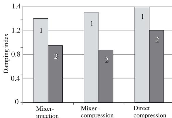
Fig. 9. Damping index of abaca fibre-PP composites in different processes (fibre content: 30 wt. %, fibre length 5 mm): 1 — without MAH-PP, 2 — with 5 wt. % of MAH-PP
