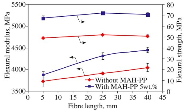
Fig. 5. Influence of fibre length on flexural modulus and strength of abaca fibre-PP composites in injection molding process (fibre content: 30 wt. %)
