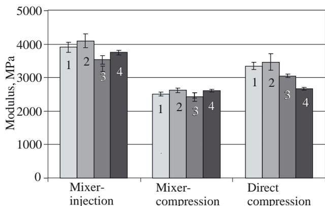
Fig. 7. Influence of compounding processes on tensile and flexural modulus of abaca fibre-PP composites (fibre length: 5 mm, fibre content: 30 wt. %): 1 — tensile modulus, without MAH-PP; 2 — tensile modulus, with 5 wt. % of MAH-PP; 3 — flexural modulus, without MAH-PP; 4 — flexural modulus, with 5 wt. % of MAH-PP
