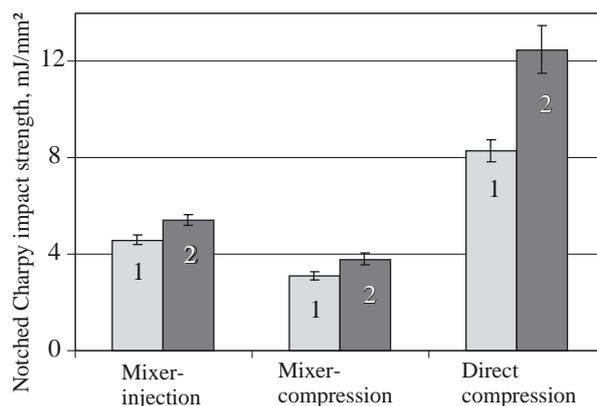
Fig. 8. Notched Charpy impact strength of abaca fibre reinforced PP composites in different processes (fibre length: 5 mm, fibre content: 30 wt. %): 1 — without MAH-PP, 2 — with 5 wt. % of MAH-PP
