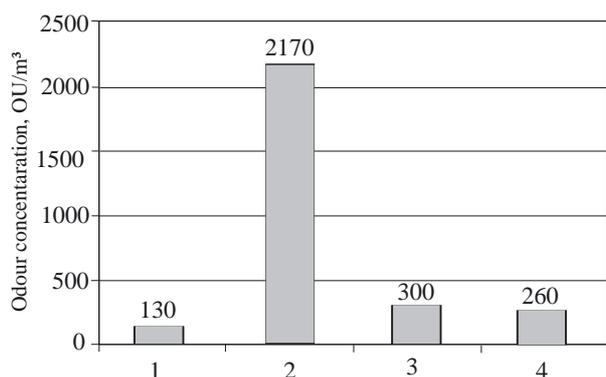
Fig. 10. Odour concentration of abaca fibre-PP composites after different processes (fibre content: 30 wt. %, fibre length 5 mm): 1 — agglomeration, 2 — agglomeration + injection, 3 — agglomeration + compression molding, 4 — compression molding
