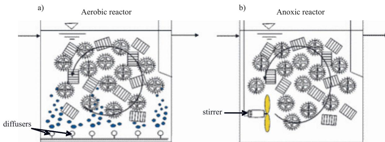
Fig. 1. Scheme showing the principle of MBBR [5]
