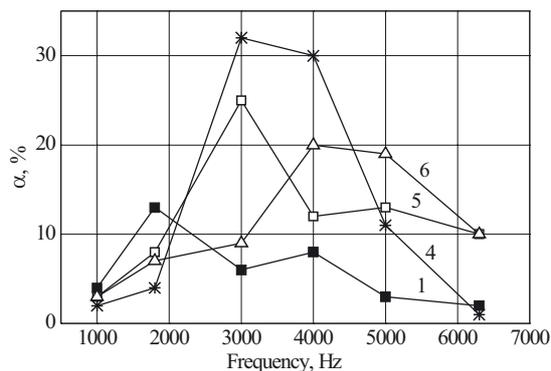
Fig. 3. Frequency dependence of sound absorption coefficient for pure polypropylene and polypropylene composites with 40 wt. % of flax, rapeseed or beech fillers; description of curves correspond to numbers of samples defined in Table 1
