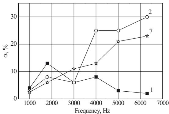
Fig. 4. Frequency dependence of sound absorption coefficient for polypropylene composites with hemp fillers; description of curves correspond to numbers of samples defined in Table 1
