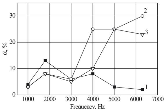
Fig. 2. Frequency dependence of sound absorption coefficient for pure polypropylene and polypropylene composites with 40 wt. % of hemp filler; description of curves correspond to numbers of samples defined in Table 1
