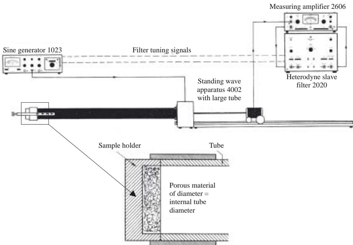
Fig. 1. Measuring setup (Standing Wave Apparatus 4002, Brüel&Kjaer) for determination of the absorption coefficient ( $\alpha$ )
