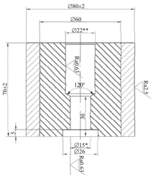
Fig. 1. Scheme and dimensions of die for the production of test samples
