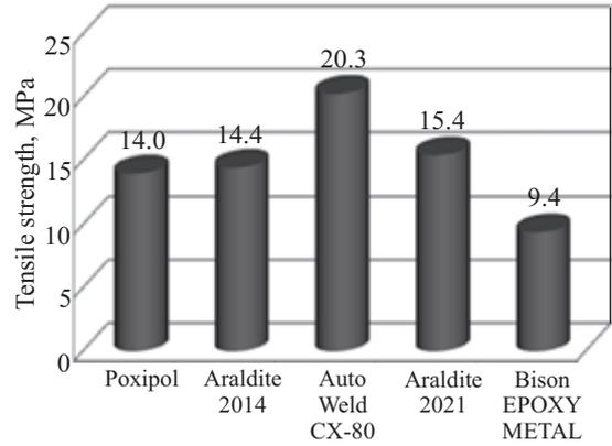
Fig. 9. Results of tensile strength tests for connected iron composite — type A from Fig. 2
