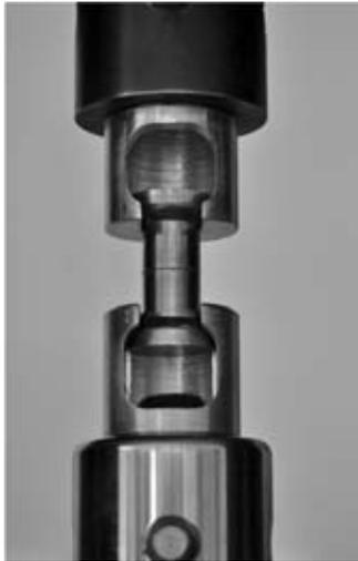
Fig. 3. A sample placed in the tensile test machine handles
