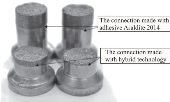
Fig. 8. Samples of type C after the strength tests
