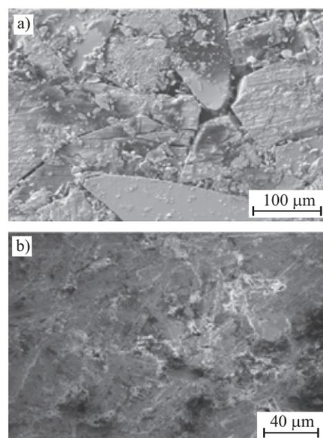
Fig. 5. SEM images of the surface: a) bonded magnet, b) soft magnetic composite
