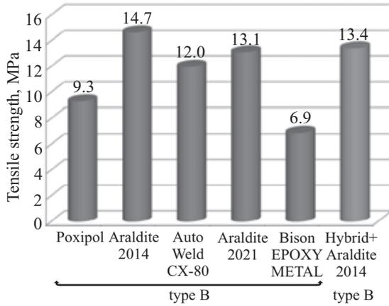
Fig. 6. Results of tensile strength tests for connected iron composite and bonded magnet — type B and C from Fig. 2
