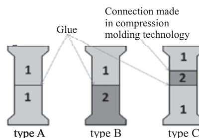
Fig. 2. Three types of tested samples; designations of materials: 1 – soft magnetic material, 2 – hard magnetic material
