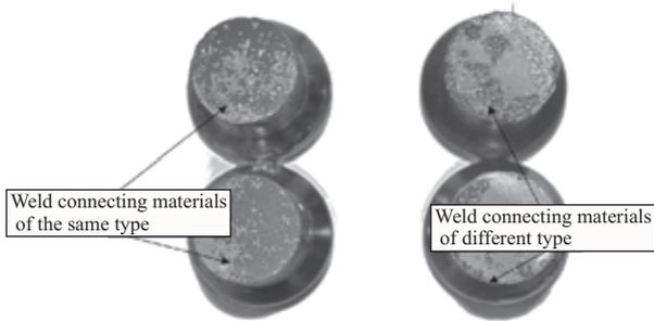
Fig. 7. The surfaces of samples after the tensile test
