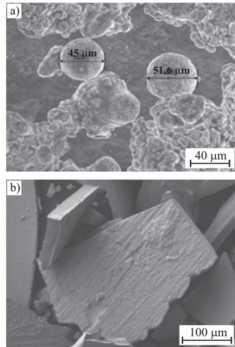
Fig. 4. SEM images of magnetic powders: a) iron powder grains, b) Nd-Fe-B grains
