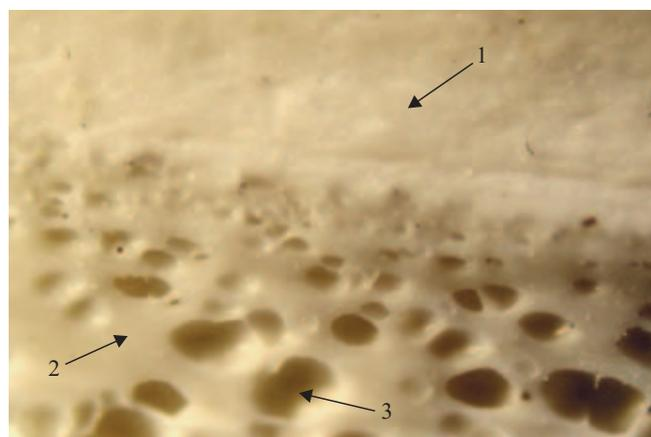
**Fig. 3.** View of double-layered coatings structure containing blowing agent in amount 0.4 wt. %: 1 – solid external layer, 2 – cellular external layer, 3 – pores
