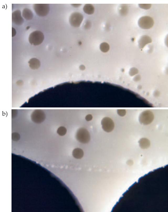
Fig. 5. Microscopic images (100× magnified) of two fragments (a and b) of the cross section obtained for single-layered coatings made of cellular PVC with 0.3 wt. % of the blowing agent
