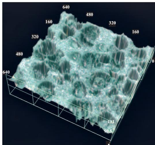
Fig. 6. Microscopic image (confocal microscope, type Olympus FluoView FV1000) of the cross section of the single-layered cable coating made of cellular PVC and 0.4 wt. % of the blowing agent
