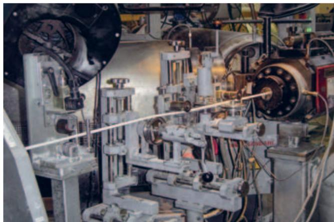
Fig. 1. Section of the technological line for cellular co-extrusion
