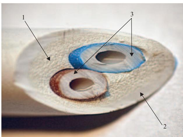
**Fig. 2.** View (20× magnified) of double-layered coating structure (copper cores have been removed) obtained using blowing agent in amount 0.5 wt. %: 1 – cellular internal layer, 2 – solid external layer, 3 – layers of cable cores
