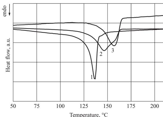
Fig. 2. DSC melting curves of the composite aged in atmosphere conditions: 1 — material not attached to the molding surface, 2 — material removed from the surface layer to the depth of about 0.05 mm, 3 — material removed from the deeper layer (from the depth between about 0.05 and 0.1 mm)
