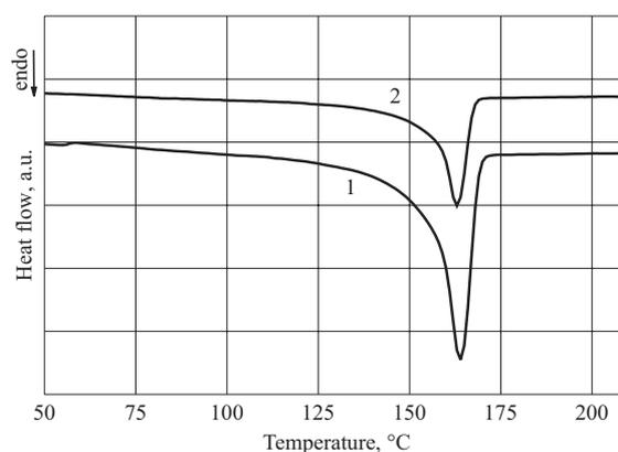
Fig. 1. DSC melting curves of: 1 – polypropylene Moplen HP548R, 2 – non-aged composite
